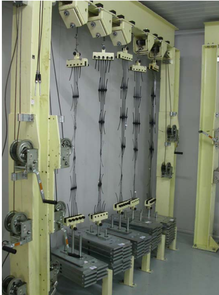
Fig. 1: Creep tests in progress at 20°C
